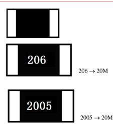
4.4 Standard E-96 series values of  $0603 \leq 1\%$ : due to the small size of the resistor's body, 3 digits marking will be used to indicate the accurate resistance value by using the following multiplier & resistance code. Multiplier Code (for  $0603 \le \pm 1\%$  marking)
